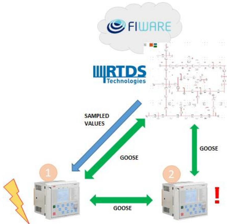
Fig. 5 Protective relays and communication schemes
