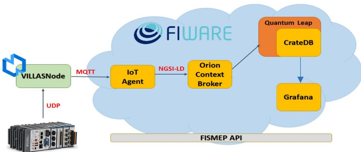
Fig. 2 Architecture of the FISMEP platform
