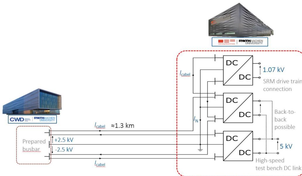
Fig. 1 Scheme of the MVDC research grid.
